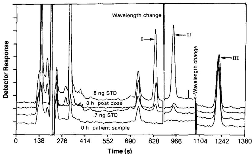
Fig. 2. Chromatograms illustrating the separation and detection of indolidan (I), its dehydro metabolite (II), and the internal standard (III) in calibration standards and in plasma from a normal volunteer administered a single 500- $\mu\text{g}$  dose.
